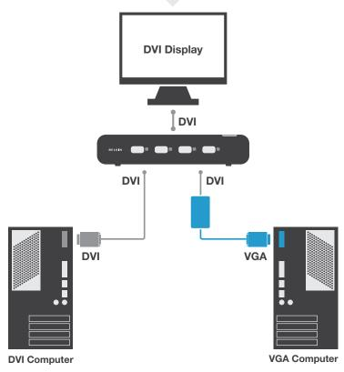
The cable converts the video signal (VGA or DVI) from the PC to a compatible signal for the KVM.
