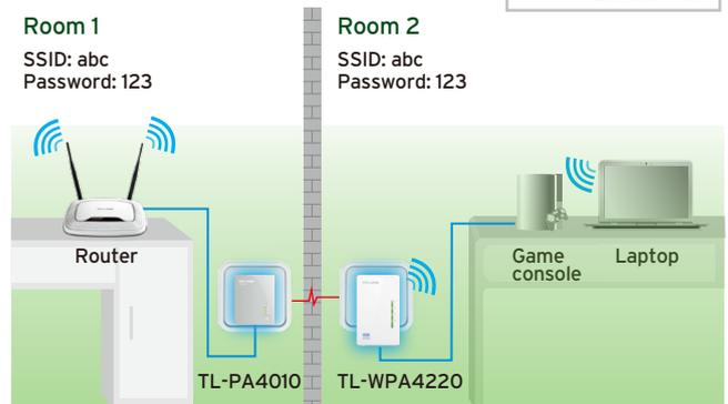
\*The Powerline Adapters need to be connected in the same electrical circuit.
