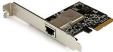
The ST10000SPEX PCI Express 10 Gbps Network Card lets you add a 10-Gigabit Ethernet port to your server or high-powered workstation through a PCI Express x4 (or higher) slot.
